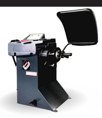
Max. wheel diameter 820 mm - Max. rim diameter 26,5" M/24"A - Max. wheel weight 65 kg - Max. rim width 20" - Electric motor and power supply 230V - 1 ph 50-60 Hz - Overall dimensions of the machine  $1100 \times 1270 \times 1280 \text{ mm}$  - Accuracy 1 g / 0.05 oz
